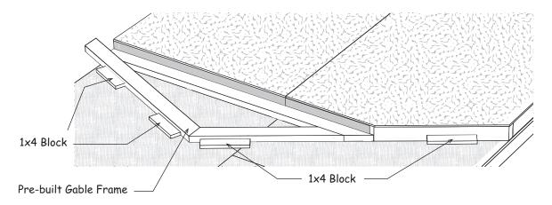
3. Position a 69-1/2" long 2x4 and a 47-1/8" long 2x4s on the floor against the 1x4 blocks and secure the 2x4s together with a wood gusset. Using (10) ten 6d common nails evenly spaced.
