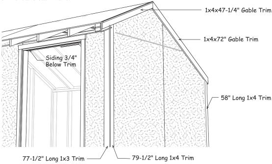
5. Install (2) two 1x3x72" boards along each side of the door opening, flush with the bottom edge of the siding. Tack these boards with a couple nails; you may want to move the trim later when you install the doors. Install a 1x3x55-1/4" board, *that has angle cuts on both ends*, across the top of the side trim. About 3/4" of siding will hang below top trim.
