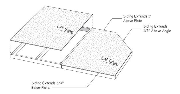
9. Position the other set of end wall frames on the floor. This time with the frame with the angle corner on the left as shown.
